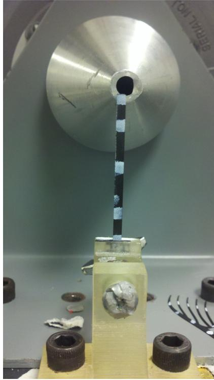
Figure 65: 40 mm x 2.5 mm beam with airhorn excitation
