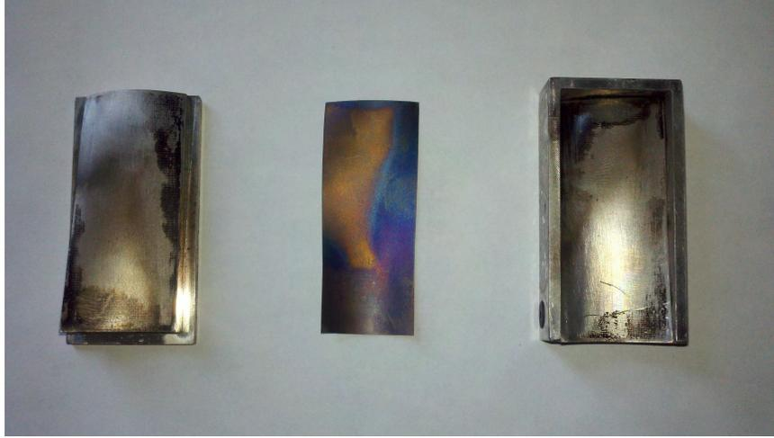
Figure 54: Machined Aluminum Mold with Sample Nitinol Sheet
