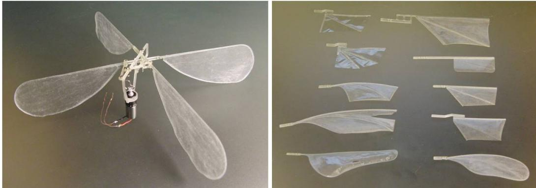
Figure 16: Flying UV Polymer Based FMWAV [75]
