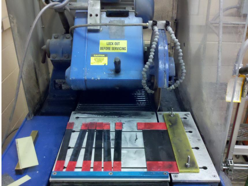
Figure 58: Coupons Being Cut In Diamond Saw
