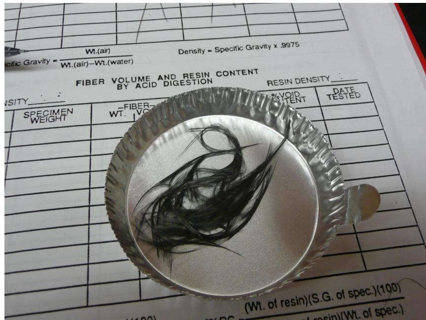
Figure 64: Recovered Composite Fibers
